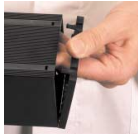
Fix the printed circuit board by settling the rear frame
