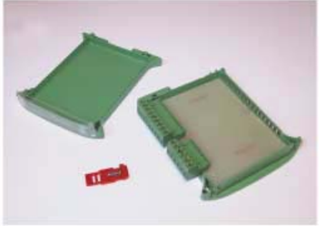
Insertion of the PCB into the base of the enclosure.
